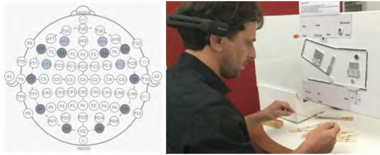
Figure 3: Emotiv EPOC+ Electrodes (10-10 I.S.) and experiment setup.
